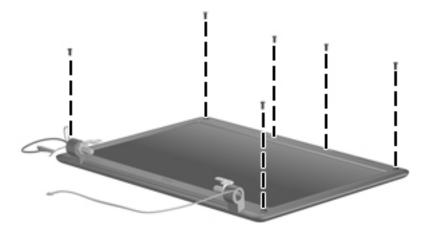
Where used: 6 screws that secure the display bezel to the display enclosure
